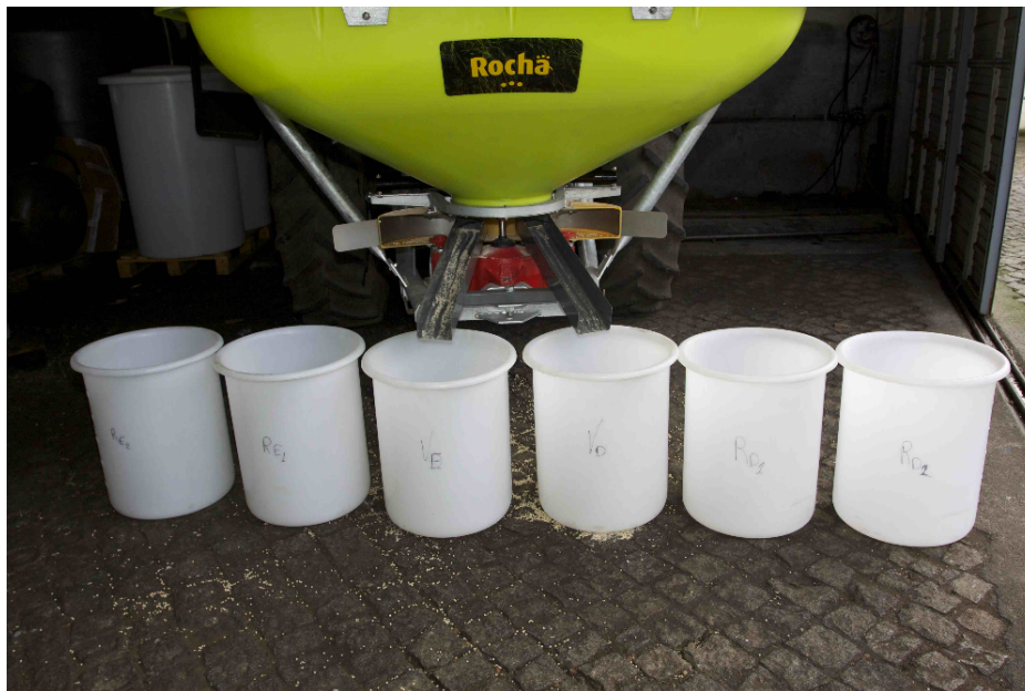
Figure 1. Fertiliser spreader prepared for the static fertiliser flow tests. Photo: Pulverizadores Rocha, SA.
